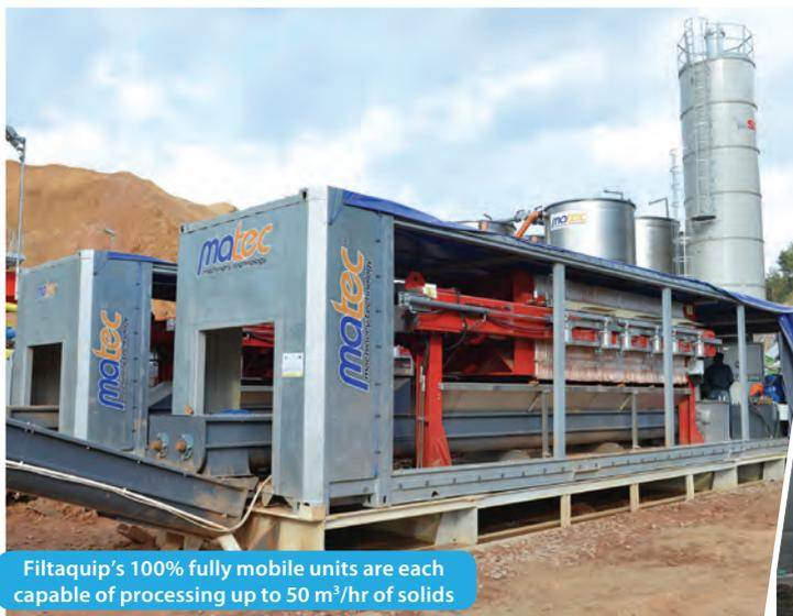
Filtaquip's 100% fully mobile units are each capable of processing up to 50 m<sup>3</sup>/hr of solids
